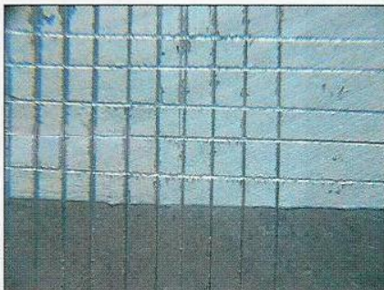
Zinga over the old phosphate system using weights of 20g/m 2 and with pull-off values of 4MPa.
