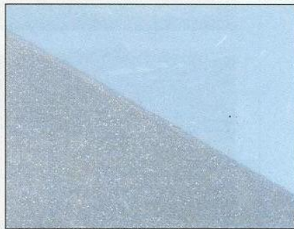
The new phosphating process with weights of 1200g/m 2 . Initial testing has shown pull-off values at around 7 MPa. The zinc is above right in the photograph and the rough phosphate is low left.
