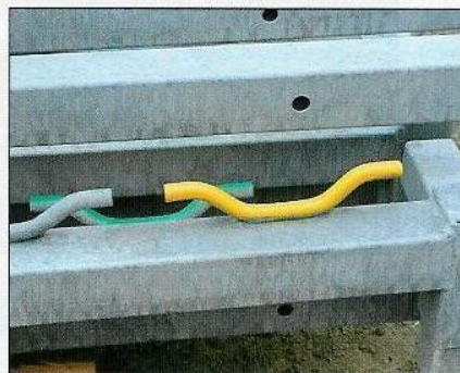
Dipped 'Zinganised' steelwork for the MoD. Note: The zinc has taken on a mottled appearance due to its early exposure to rain soon after being coated. This is very good for the coating's morphology.
