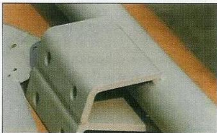
Tow-bars cold-galvanised with 'Zinga'. These units would normally be finished with a wet coating such as a 2K polyurethane.
